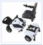
Dismantles easily into 3 pieces to fit in a car boot for transportation
